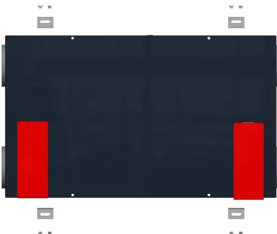
Fig. 9: Attaching the mounting brackets
