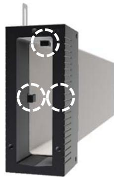
2. Shorten the flat duct (6) by the determined length so that the area of the recess grooves or at least the front side of the duct adapter (8) is located in the planned final facade finish of the vertical window reveal.
